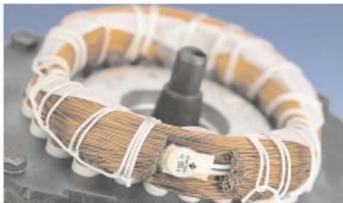
The thermal protections, connected singularly or in three groups within the windings of the stator, detect their temperature of exercise and switch-off the contact when the detected temperature achieve up to the set value for which they have been constructed within a tolerance of  $\pm 3\%$ . The thermal sensors start, once well connected to the control panel, safeguard motor from the risk of overloading and eventual burning.
